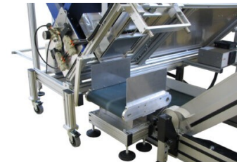
Picture 5: LQX100 Checking of finished bags before conveyor belt
