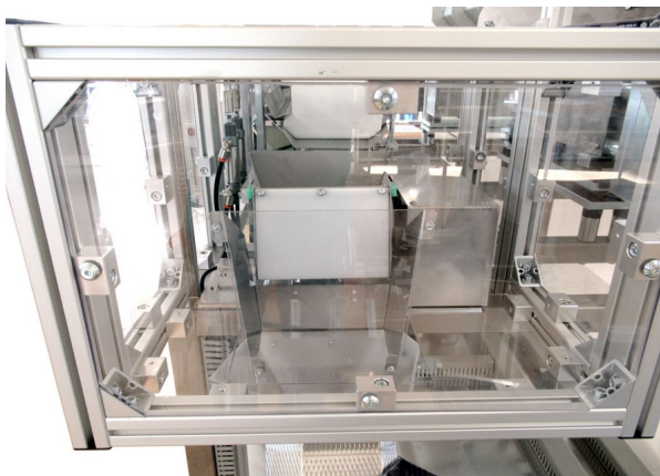
Picture 5: The weighing hopper is protected from external influences by a housing. As a result, in addition to noise reduction, counting accuracy is increased.
