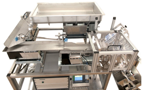
Picture 6: Compact design of a LZ100 complete system with good accessibility. The installation and arrangement is individually adapted to your needs.
