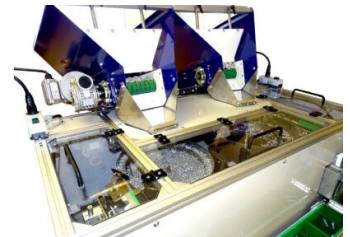
Picture 4: 2-pot bowl feeder system with bunker and noise protection cover (accessible from the top)
