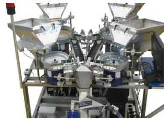
Picture 3: 4-pot bowl feeder system with bunker and customized feeding system into the filling funnel.
