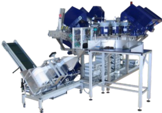
Picture 1: 7-pot bowl feeder system with bunker, sorting table, conveyor belt, and other add-on components
