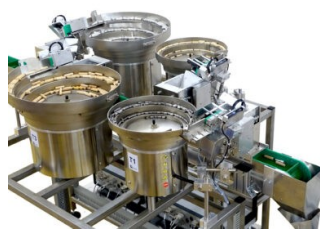
Picture 2: 4-pot bowl feeder system with collecting belt to convey the counted parts to the LVX packaging machine.
